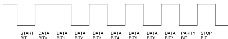
Fig 20.1 – Timing diagram for a serial character
