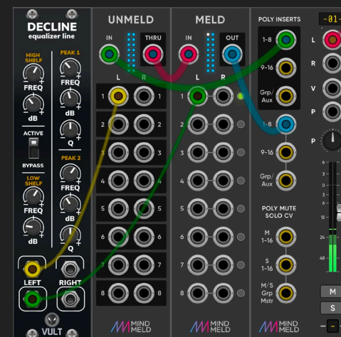
Adding an EQ on Track 1 using our Meld and UnMeld utilities – much less patching required!
